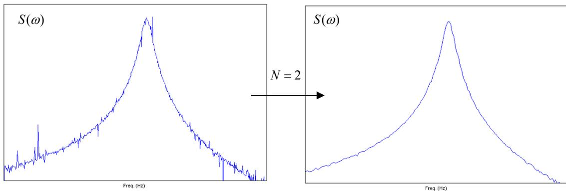
**Fig. 10 - Frequency Averaging of Spectral Density Functions**
