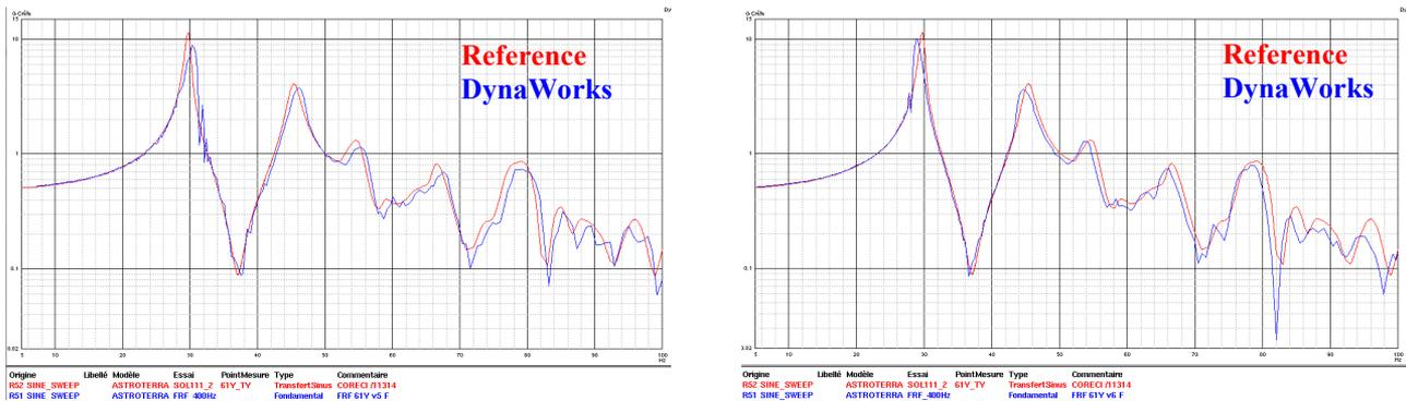
Figure 21 - FRF using DynaWorks Method
