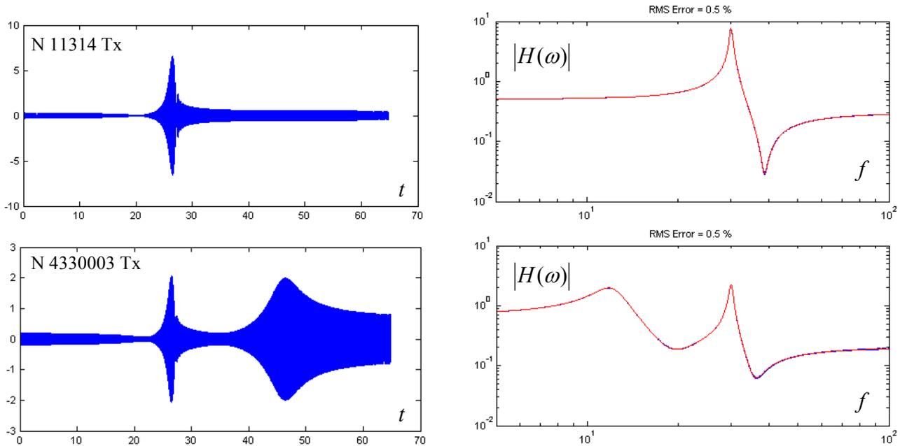
**Fig. 15 - FRF using Wide Band Method on SPOT 6 Condensed Model**
