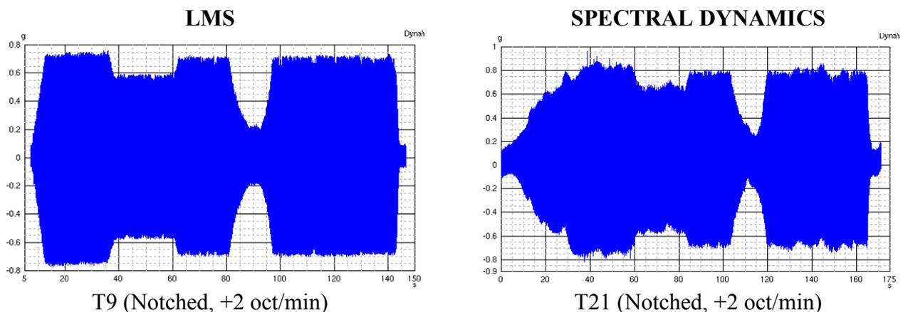
**Fig. 7 - Comparison of Sine Sweep Inputs**
