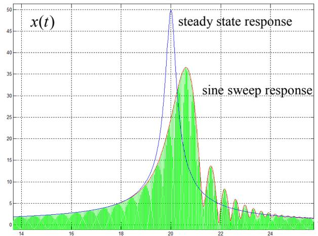
**Fig. 2 - Effect of Sine Sweep on SDOF Response**
