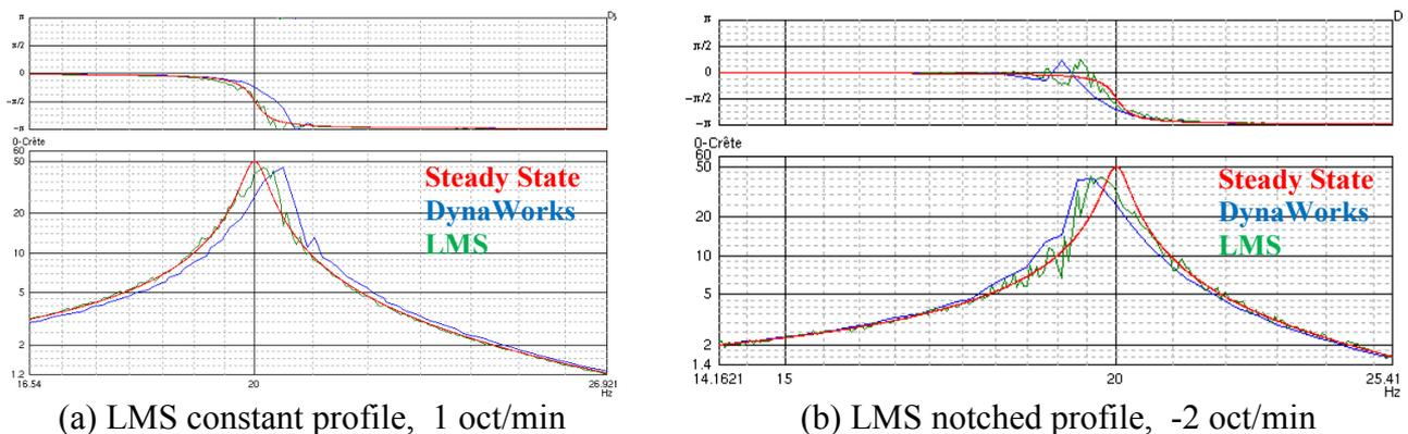
**Fig. 12 - Comparison of FRF obtained from DynaWorks and LMS**
