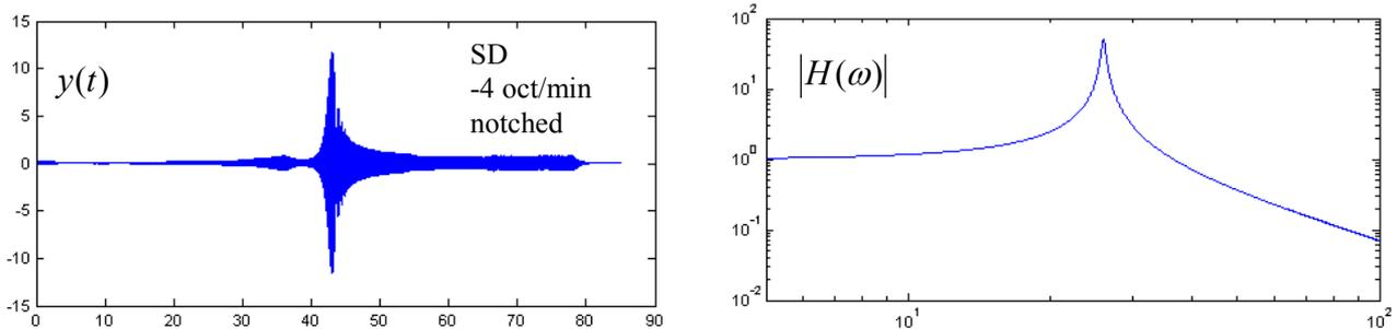
**Fig. 13 - FRF using Wide Band Method on SDOF Model**
