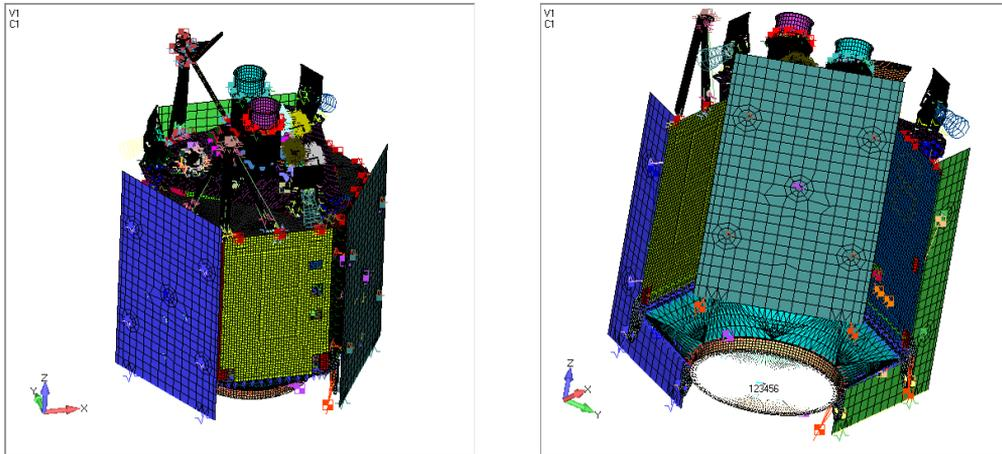
**Figure 20 - SPOT6/ASTROTERRA FEM**
